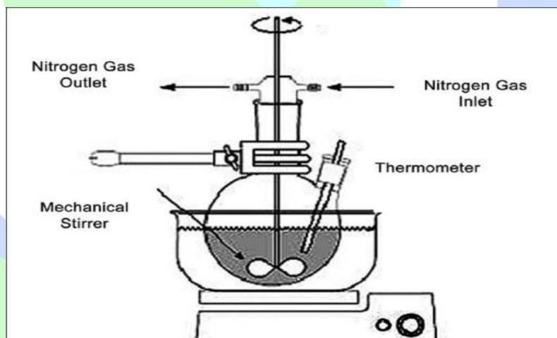
**Fig.2: instrument set up for suspension polymerization technique**
